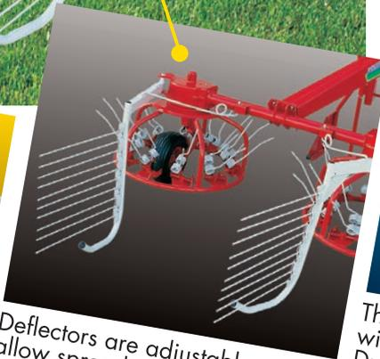
Deflectors are adjustable to allow spread turning of hay when they are wide open. They can be closed following working needs to obtain even and aerated windrow.
