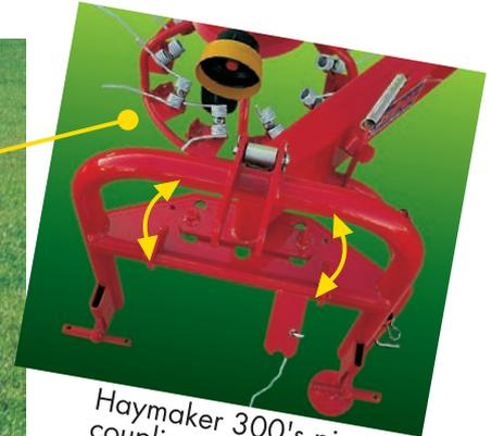
Haymaker 300's pivoting coupling allows the machine to follow tractor's course thoroughly. When the Haymaker 300 is lifted it locks automatically on center position in order to avoid lateral oscillation. Machine locks also on uneven grounds.
