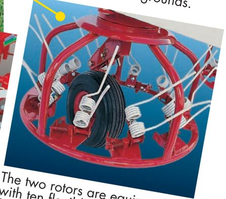
The two rotors are equipped with ten flexible tines each. During operation, tines are set level due to centrifugal force. To obtain perfect turning and windrowing, one tine out of two, provides wider opening to increase the worked area and to allow passage in very thick hay.
